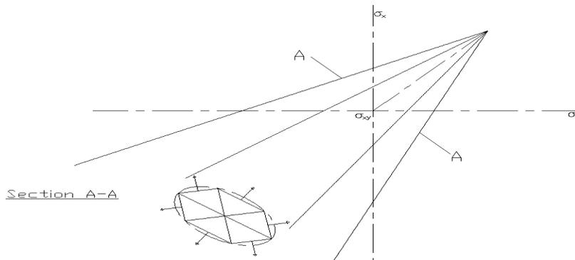
Fig (2): Piecewise Linearized Mohr-Coulomb Yield Surface in Plane Strain, Anderheggen [12]
