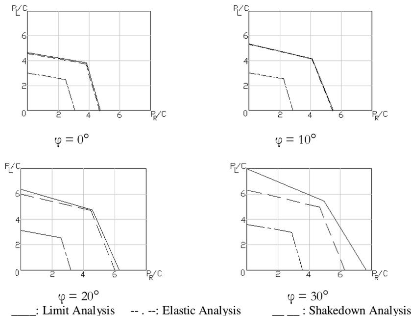
Fig (3): Elastic, Shakedown and Limit Domains for the field Problem at different angles of internal friction
