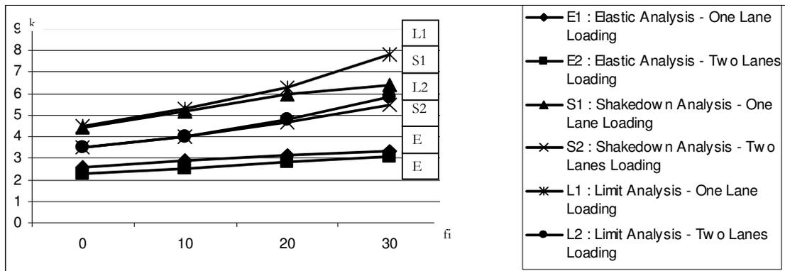
Fig. (4): Elastic, Shakedown and Limit Load Factors Due to Different Loading Programs and at Different Angles of Internal Friction.
