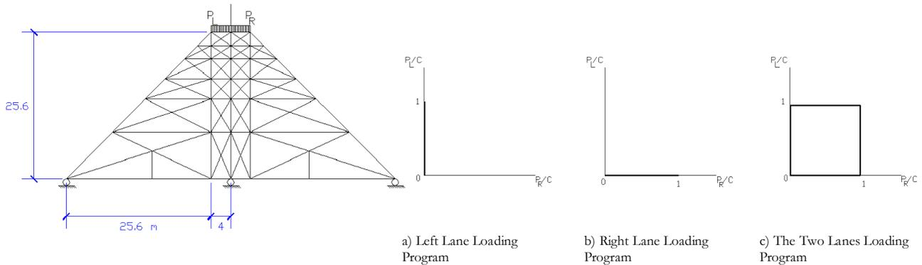
Fig (1) Finite Element Discretization for the Field Problem and Loading Programs, (PL and PR are traction loading and C is the cohesion).
