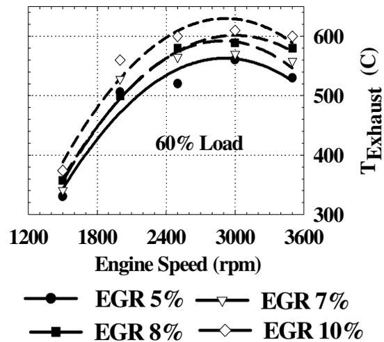
Fig.(11)  $T_{\text{Exhaust}}$  for Different EGR with 60% Engine Load
