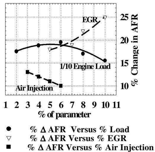
Fig. (9) Effect of Load, EGR and Air Injection on Percentage Change of AFR
