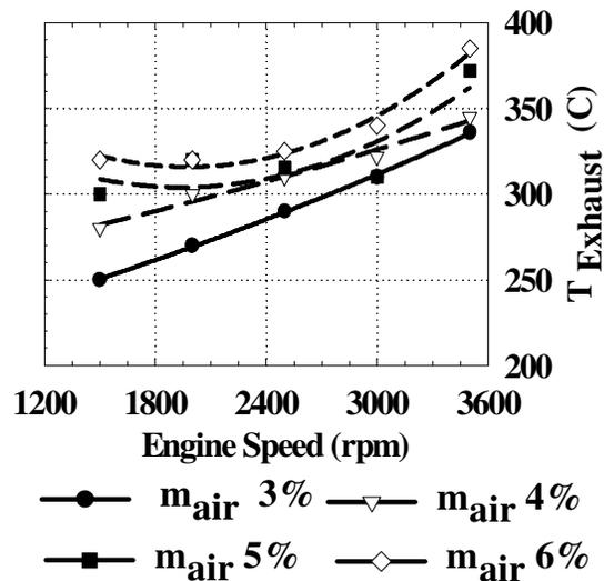
Fig.(13)  $T_{\text{Exhaust}}$  for Different Percentages of Air Injection at 60 % Load
