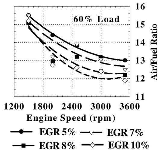
Fig. (7) Air/Fuel Ratio for Different EGR
