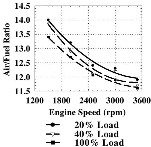
Fig. (6) Air/Fuel Ratio for Different Engine Loads
