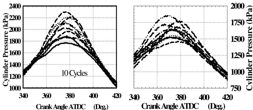
Fig.(20) Cycle to Cycle Variations of Cylinder Pressure at Speed of 1500 rpm and 60% Load
