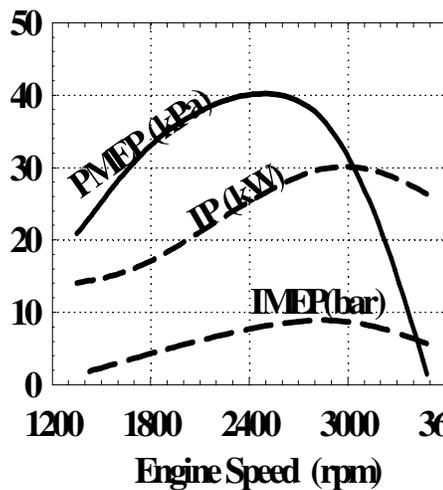
Fig.(4) IMEP, IP and PMEP at 100% Load
