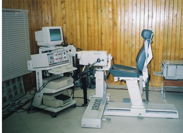
**Fig.1\*Biodex Isokinetic dynamometer**
